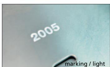
By applying of anticorrosion electrolyte on the screen printing form it is possible to autographe durable manufacturers logo's, serial numbers etc. on metal surfaces for example type plates and tools.
